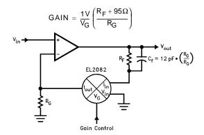
FIGURE 4. EL2082 IN FEEDBACK NON-INVERTING GAIN
