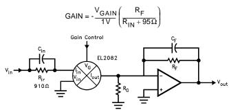
FIGURE 2. INVERTING EL2082 + OP-AMP
