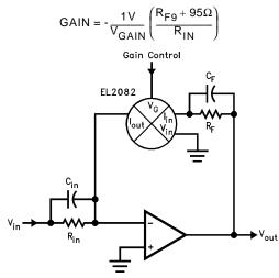
FIGURE 3. EL2082 IN FEEDBACK INVERTING GAIN
