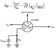
FIGURE 5. THE VIN PIN USED AS SIGNAL INPUT
