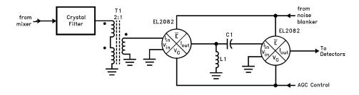
FIGURE 7. EXAMPLE REACTIVE COUPLINGS WITH EL2082'S
