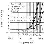
**Output Current Noise** vs Frequency
