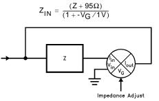
FIGURE 11. VARIABLE OR NEGATIVE IMPEDANCE CONVERTER
